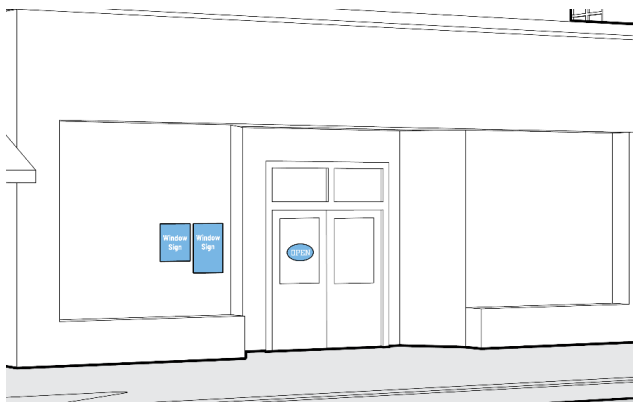
Figure 54: Signs should not obscure the transparency of windows.
