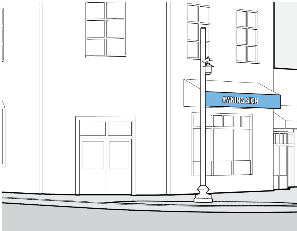
Figure 57: Awning signs with lettering located on the front flap of the awnings are encouraged.
