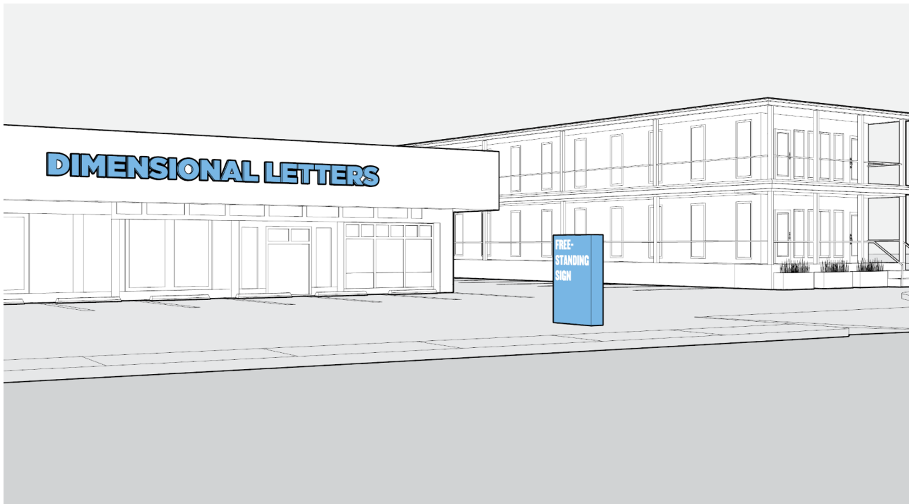
Figure 28: Illustration of permitted signs in vehicle-centric areas, including free-standing signs and dimensional lettering directly mounted on the building.
